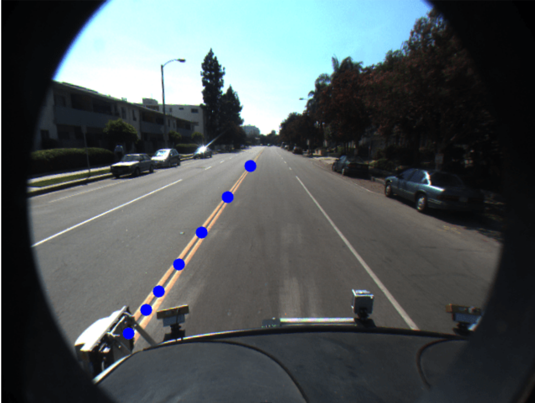
Automatically Marked Lane Boundary Points
