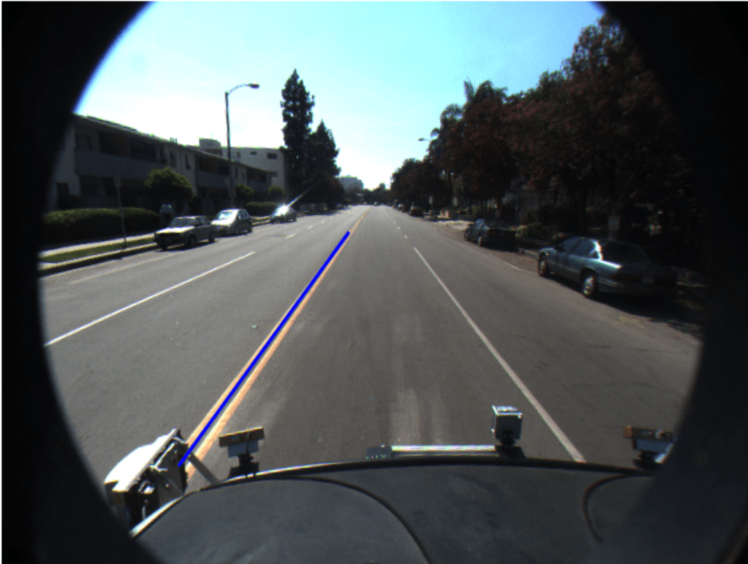
Detected Left Lane Boundary Model
